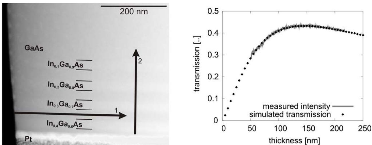
Fig. 1. a) HAADF STEM cross-section image of wedge-shaped sample at 25 keV. b) Comparison of the measured intensity along the GaAs layer with simulated electron transmission as a function of the sample thickness.
