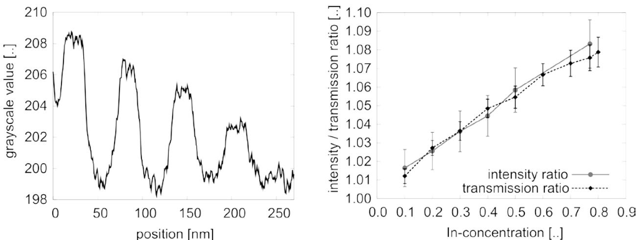
Fig. 2. a) Intensity linescan across the  $\text{In}_x\text{Ga}_{1-x}\text{As}/\text{GaAs}$  QW structure. b) Comparison of measured intensity ratios with simulated transmission ratios as a function of the In-concentration.
