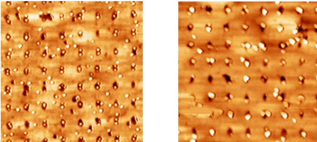
Fig. 1: AFM images ( $2\ \mu\text{m} \times 2\ \mu\text{m}$ ) of two samples with InAs QDs grown on patterned GaAs substrates. (Left) Sample with 1.7 ML InAs coverage. Double dot nucleation per hole is predominantly observed. (Right) Sample with 1.7 ML InAs coverage, annealed for 2:30 min. One dot per site is found in most cases.
