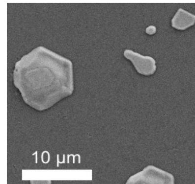
Fig. 1: Cu-doped GaN with Cu-Ga islands on top of the surface
